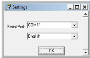
3. Choose the command **Settings** in the menu bar and select in the **Serial Port** list the port to which the module is connected. Press the button **OK**.
