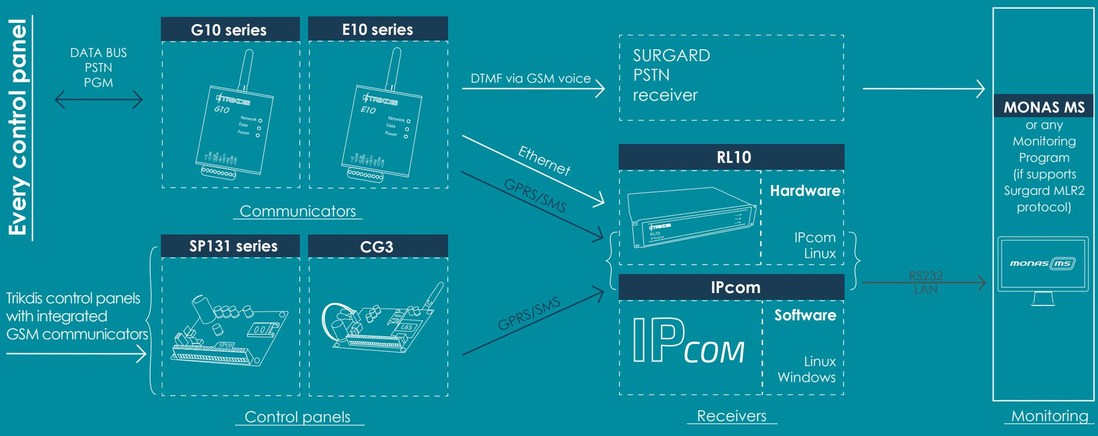
**Fully compatible.** Our G10 and E10 series communicators transfer full alarm information from the majority of security control panels on the market, therefore it is easy to integrate TRIKDIS communicators into an existing security system. Data Bus compatible with: **Paradox, DSC, Pyronix, Caddx, Crow, Texecom.**
