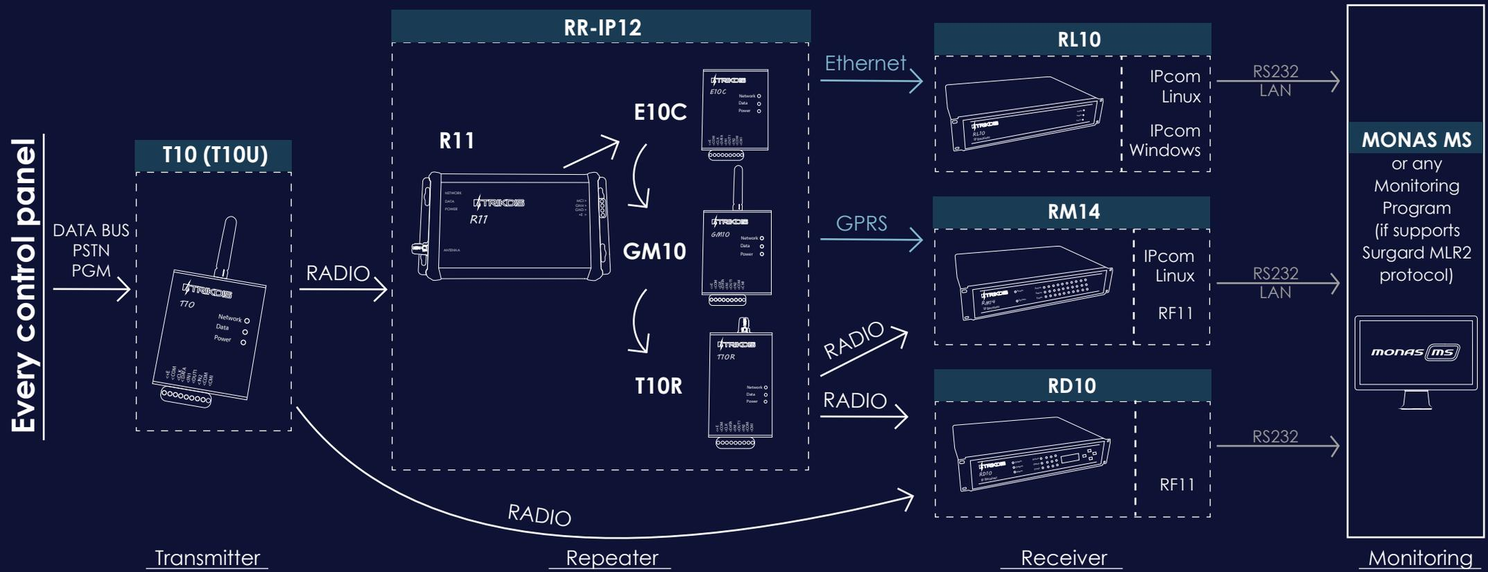
**Communications network can be created in VHF or UHF radio band.**
