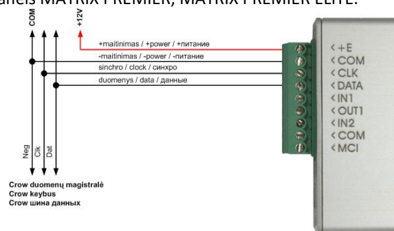
Transmitter T10R ( T10UR ) connection to Texecom control panels MATRIX PREMIER , MATRIX PREMIER ELITE .
